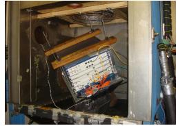
Network Blade on Quanta's ED Shaker/Chamber with Skewed Fixture
